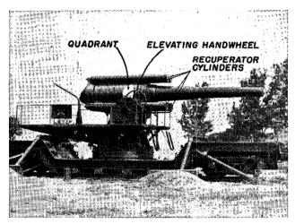
FIGURE 4.—8-inch gun in firing position.
